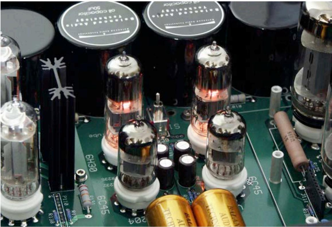
They incorporate two types of vacuum tubes, user selectable for the desired sound: 6C45 and 6H30.
