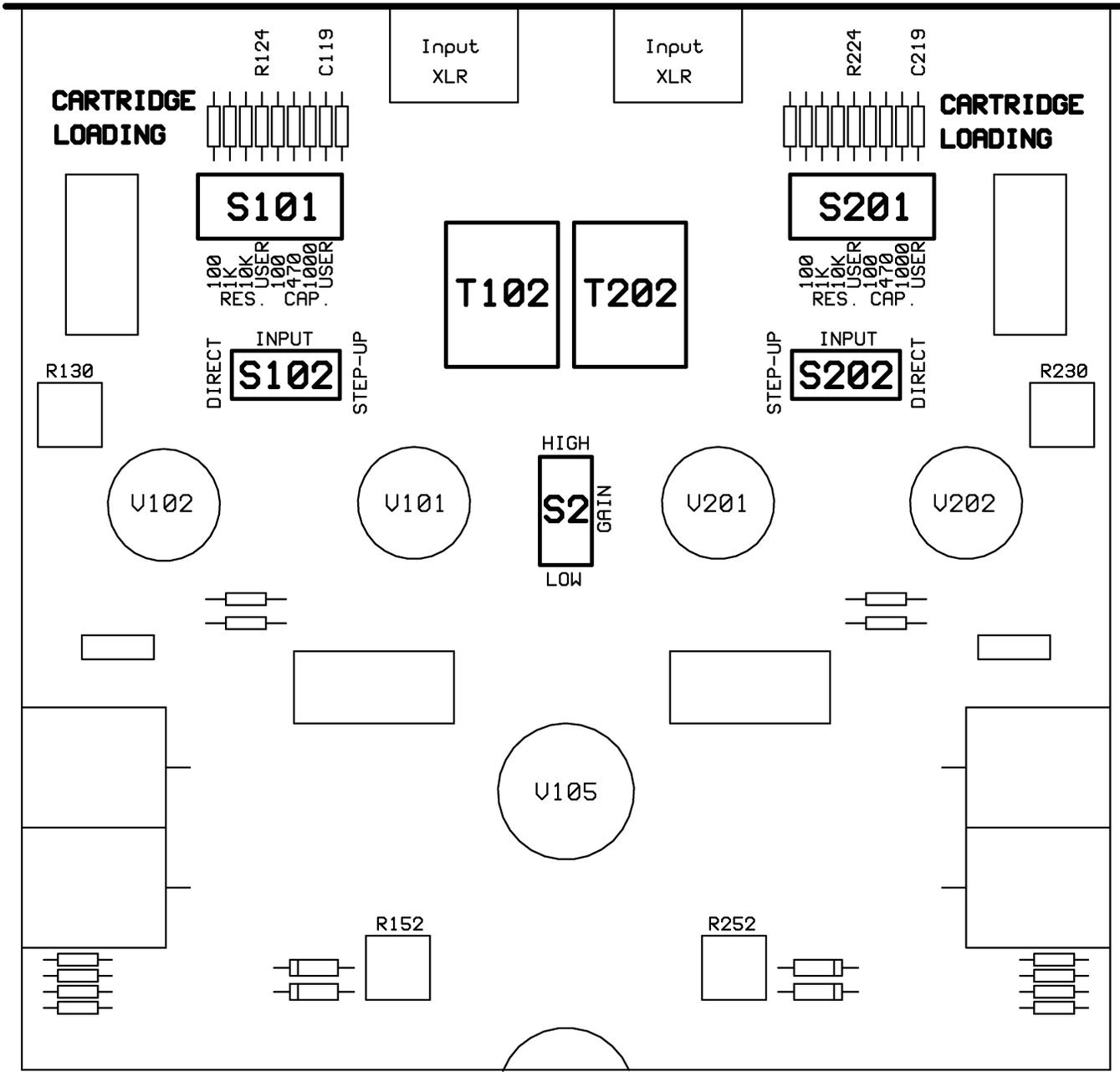
Figure 1: UK-P10 Internal Controls
